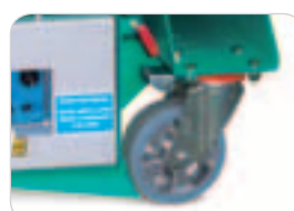
Swivel castor interlock for straight line driving.
